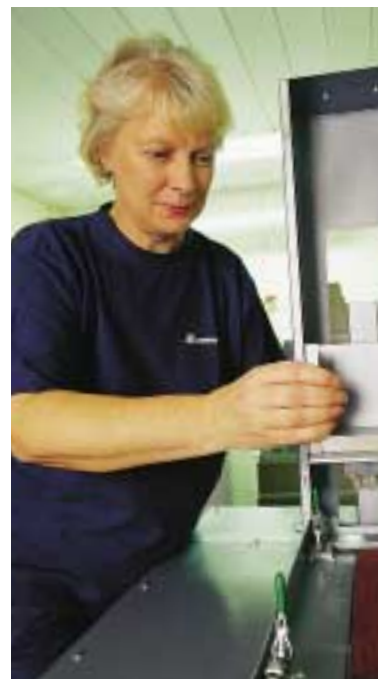
Laboratory technician Airi Leikas tests the chippings of a bituminous sheet membrane in the Company's Central Laboratory.
